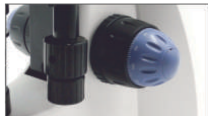
Coaxial coarse & fine focusing, with tension adjustment. Fine division 0.002mm, coarse stroke 36mm
