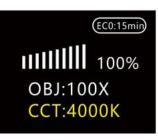
Long press the dimming hand wheel to adjust the color temperature interface 3000K-7000K
