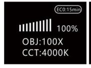
ECO duration, lighting brightness, objective magnification, and color temperature are displayed on the working screen.
